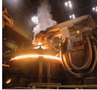
Aqualoy shafting starts with careful selection of raw materials combined and melted in an electric arc furnace.
