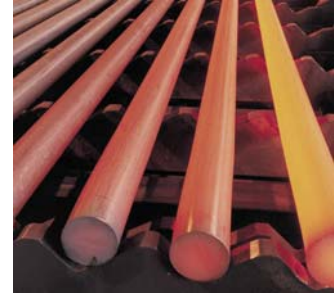
After rolling with precise temperature and reduction control, hot/cold worked shafting is shown on the cooling bed.
