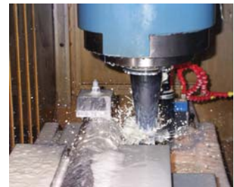
CNC milling of keyway, a value-added service to our distributors.
